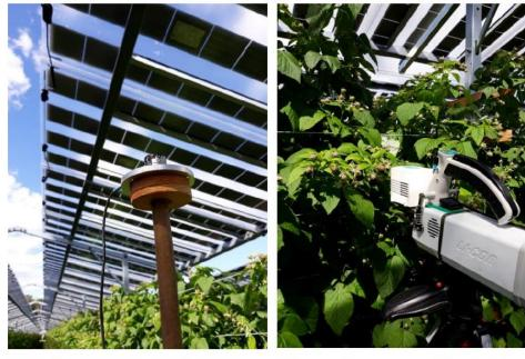
Figure 4. PAR sensor below solar panels
