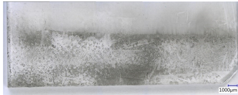
Microscope slide with PIB residues after flash lamp annealing.
