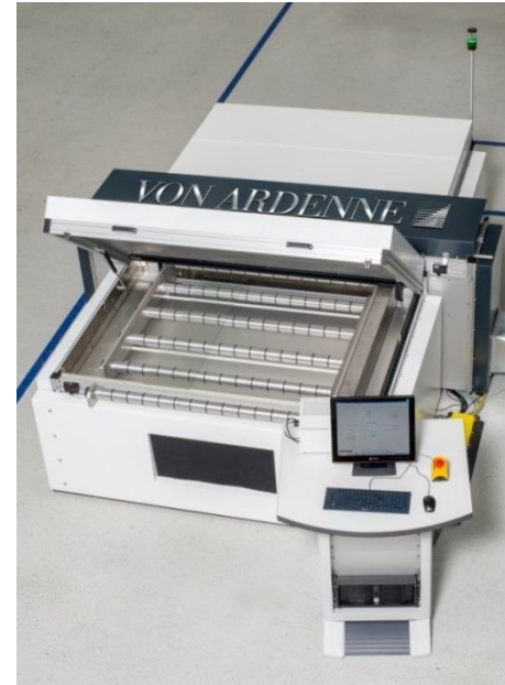
Flash lamp annealing device Credits: Von Ardenne, Germany
